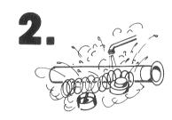
Remove spring and cup holder., Wash all parts with warm soapy water to remove dirt and wax build up. Do not bend the adjustment clips by hand.
