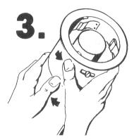
Turn collar counterclockwise until adjustment clips hold cups firmly in place. Tighten locking screw. DO NOT BEND CLIPS BY HAND!
