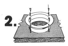
**Fasten mounting ring** securely over hole with the supplied mounting hardware.
