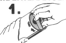
Remove spring assembly by rotating plastic base clockwise until tabs are released from window. Pull bottom out carefully.
