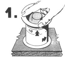
Remove dispenser from counter by rotating counterclockwise and pulling from hole.
