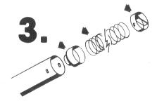
Reassemble unit by inserting cup holder, spring and bottom, making sure tabs snap into windows. Be sure to check adjustment before reinstalling.
